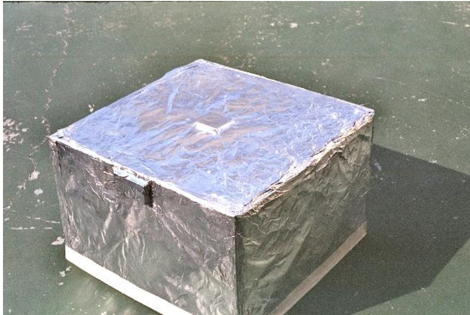
Picture 04: Verification of Robert Wood's Experiment - 1st Phase. Aluminum foil wrapped around the outside
