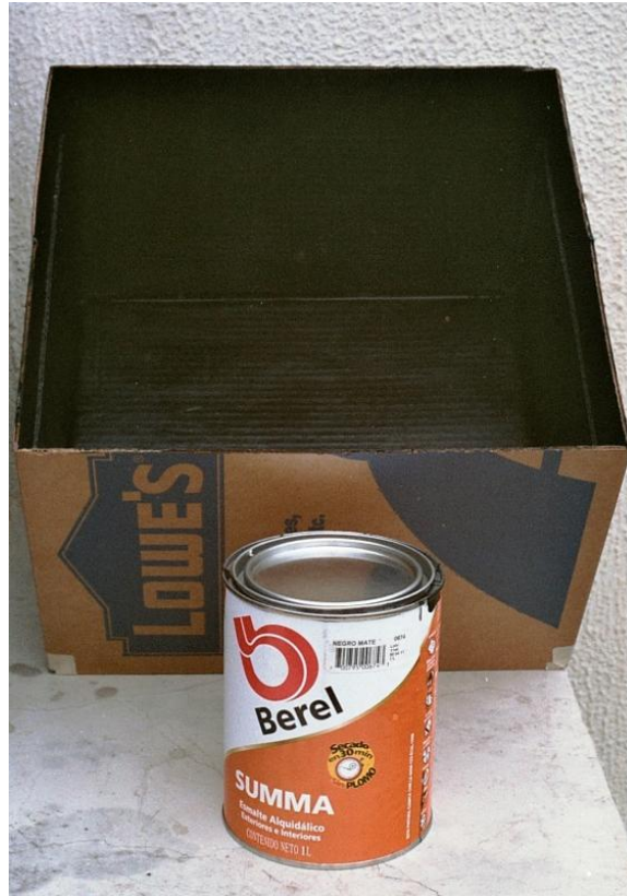
Picture 02: Verification of Robert Wood's Experiment - 1st Phase. Interior painted with Berel matt-black paint
